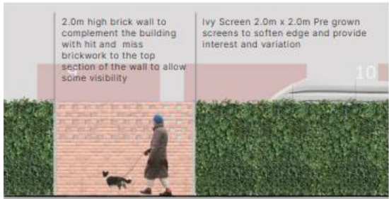
FIGURE 277. Elevation of boundary treatment - Interim
